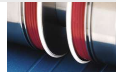
Spine & Hinge Creaser Close proximity creasing solution for perfect bound books.
